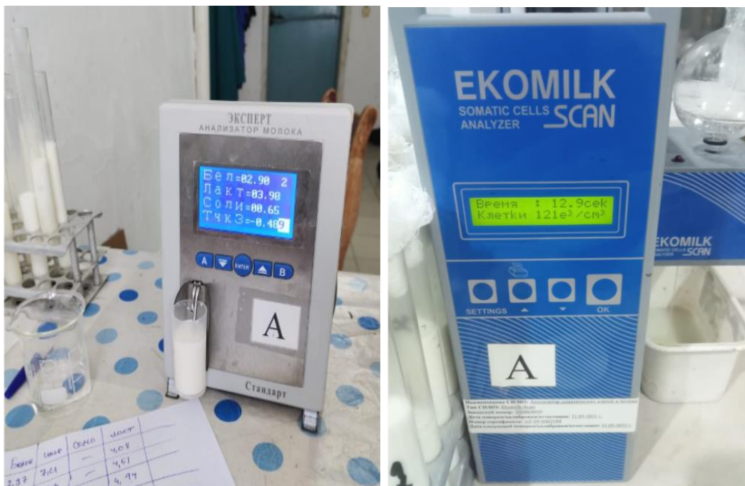
Fig.2 – Expert milk analyzer (Fig.2 – left) and somatic cell analyzer Ecomilk Scan (Fig.2 – right)
