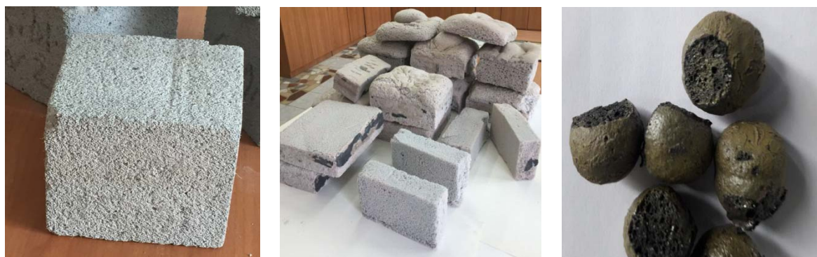
a) b) c) Picture 1 - Energy effective materials: a) foam concrete; b) foam glass; c) expanded clay
