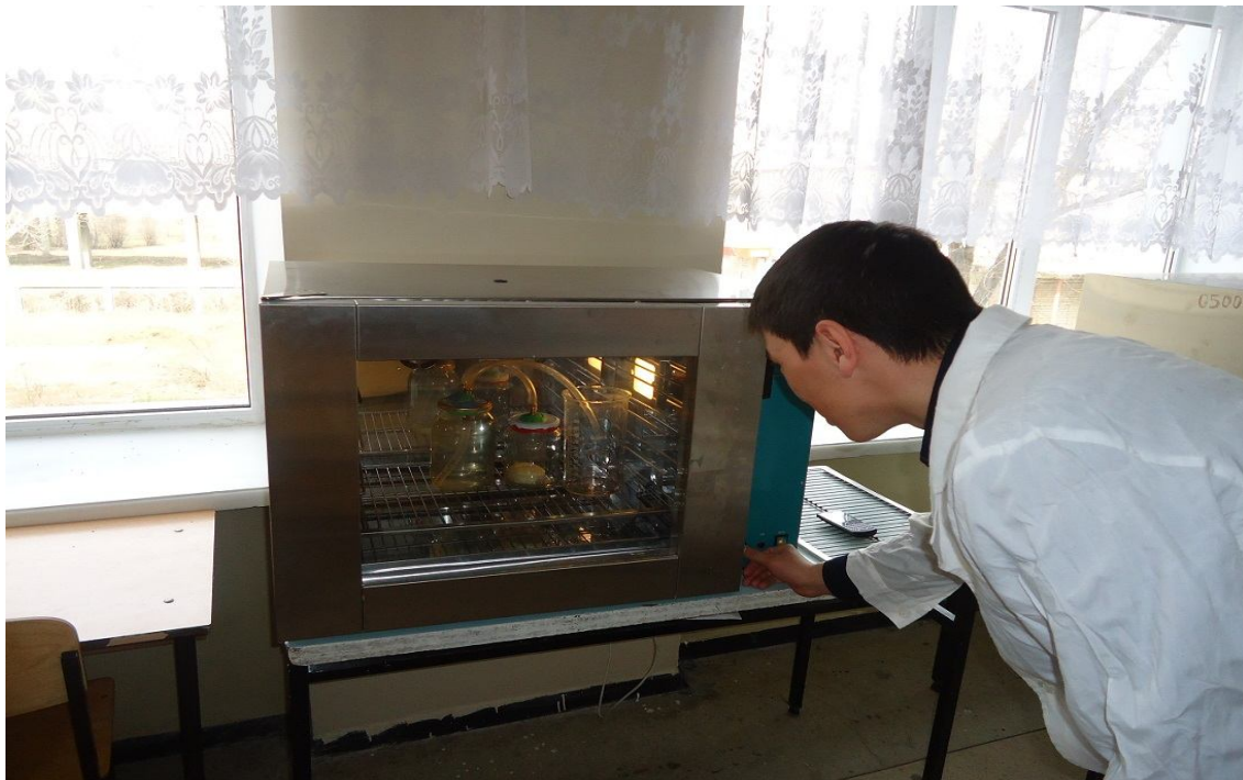
Picture 1 –Supervision of gas-forming ability of dough with the use of Brássica nápus flour by Iago-Ostrovsky designed modified device
