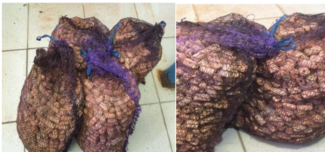
Figure 2- General view of a pilot-industrial batch of organic-mineral ceramic biomaterial of our own production made on the basis of the scientific and educational-production center of the Research Institute «Engineering and Resource Saving» Zhangir Khan WKATU.
